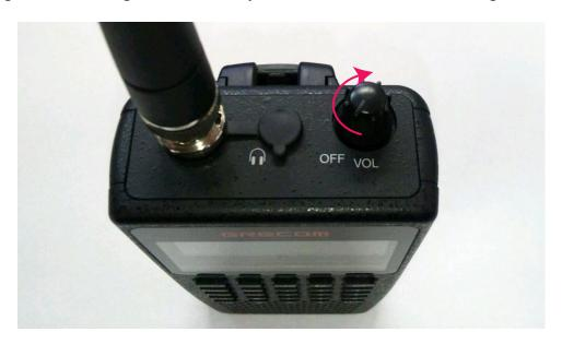
2. Press **SQ ON/OFF** switch. appears when the scanner's squelch is turn on. Select **SQ HI** or **SQ LO** if possible.
