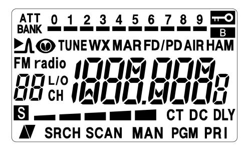
Appears when the scanner functions 20 dB attenuator.
