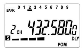
2. Press CT/DC. Ct dC-Srch appears and CT/DC flashes. Press ENT to store CTCSS/DCS code search setting into this channel.
