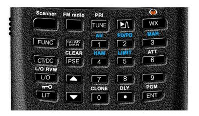
**Scanner** Return to scanner mode from FM radio mode.
