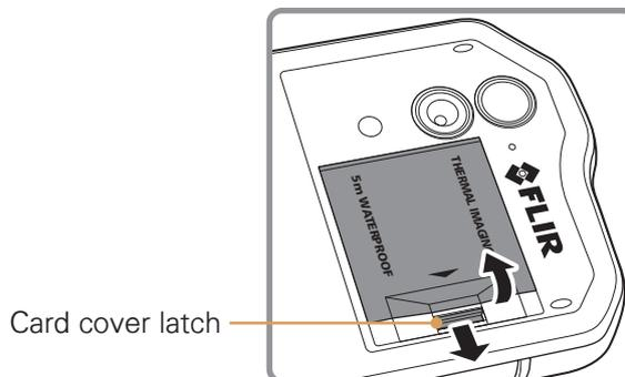
2. Insert a microSD card into the memory card slot with gold contacts facing down.
