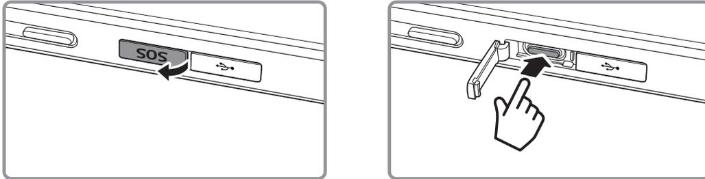
By default, the SOS key will allow you to send a predefined custom SMS message, including your current location, to up to three predefined contacts through the **Location Alert** app, installed on the device. But before the key can be used to send messages, you need to define the custom message content and who you would like to receive the message(s).
