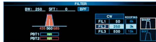
Digital IF filter setting screen
