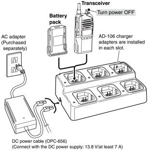
(Connect with the DC power supply; 13.8 V/at least 7 \*Abou the OPC-656 Red line :(-) Black line :(-)
