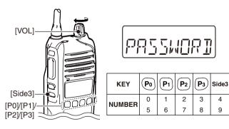
③ When the "PASSWORD" indication does not clear after inputting 4 digits, the input code number may be incorrect. Turn the power off and start over in this case.
