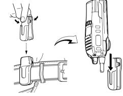
(5) Once the transceiver is locked in place, it swivels as illustrated below.
